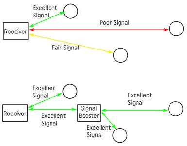
Also note that the signal degrades mainly as it passes through objects, rather than distance. So "Halfway" may not be halfway distance wise. Eg if The Thermostat to Receiver signal had to pass through 4 walls, the repeater should most likely be placed so that there are TWO walls between Receiver and Signal booster, and TWO walls between Thermostat and Signal Booster.
