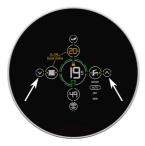
To reset the Ignite Touch Thermostat, press and hold the up and down arrows for 30 seconds. First 'C1' will display, keep your fingers held in the same position until the regular screen returns.
